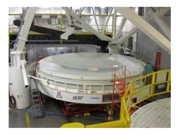
The unique primary mirror with the integrated tertiary mirror in its center will form the heart of LSST. Credit: SOML/LSST Corp
