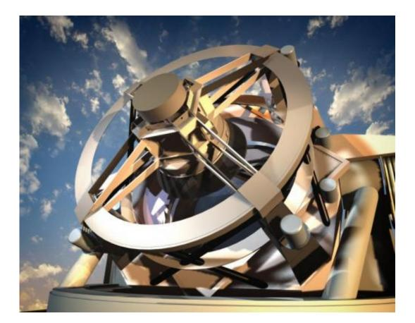
A rendering of the telescope assembly. The UA design allows for a very compact instrument, allowing it to move around quickly as it scans the sky repeatedly. Credit: Mason Productions Inc./LSST Corp.
