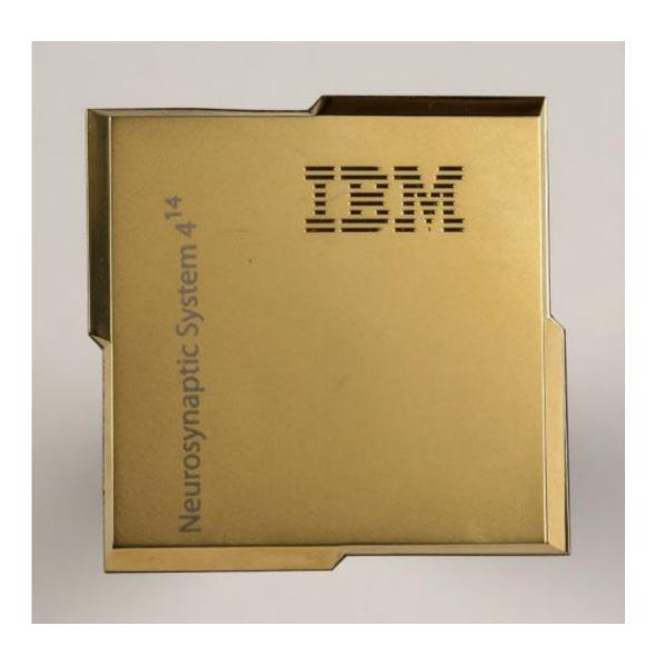
IBM's new neurosynaptic processor intergrates 1 million neurons and 256 million (414) synapses on a single chip. Credit: IBM
