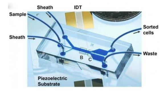
A schematic illustration of working principle and device structure for a tiltedangle standing surface acoustic wave-based cell-separation device. Credit: Tony Huang, Penn State
