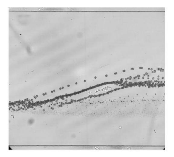
This image shows the beginning of separation stream separating cancer cells from red blood cells in the tilted-angle standing surface acoustic wave-based cellseparation device. Credit: Tony Huang, Penn State
