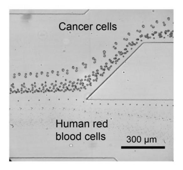
This image shows the end portion of separation stream separating cancer cells from red blood cells in the tilted-angle standing surface acoustic wave-based cellseparation device. Credit: Tony Huang, Penn State
