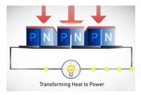
This image shows the inside of GMZ Energy's TEG module. When waste heat enters the top of the module, and moves through the semiconductor material (shown here as P and N) to the cooler side, the resulting temperature difference creates a voltage that's extracted as electricity. Credit: Screenshot from a video by GMZ Energy
