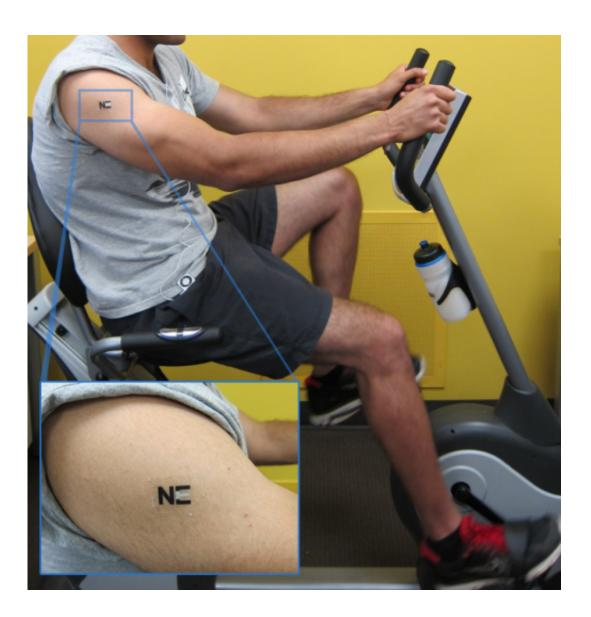
A tattoo biosensor (enlarged above) detects lactate levels during exercise; a biobattery using the technology could power electronics. Credit: Joseph Wang
