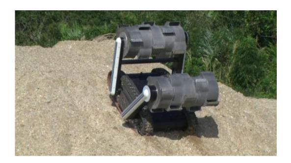
The prototype mining robot called RASSOR will be incorporated into the "swarmie" tests to see how well the software translates to different robotic vehicles. RASSOR is a concept robotic vehicle evaluating designs for a future craft that could work on another world. Credit: NASA
