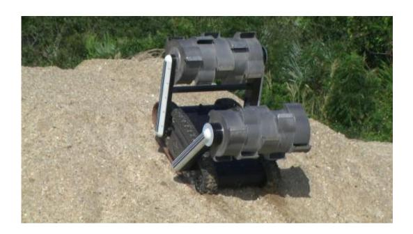
The prototype mining robot called RASSOR will be incorporated into the "swarmie" tests to see how well the software translates to different robotic vehicles. RASSOR is a concept robotic vehicle evaluating designs for a future craft that could work on another world. Credit: NASA
