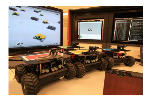
The four "Swarmies" robots on a table with the software simulation used to develop the program to control the robots. Credit: NASA/Dmitri Gerondidakis
