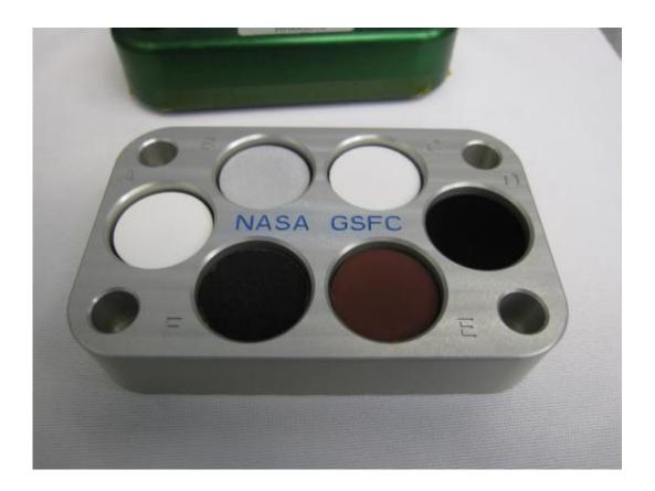
A new carbon-nanotube coating is one of several materials to be tested on the International Space Station as part of the Materials Coating Experiment. The super-black material occupies the "D" slot on the sample tray. Credit: NASA/Bill Squicciarini
