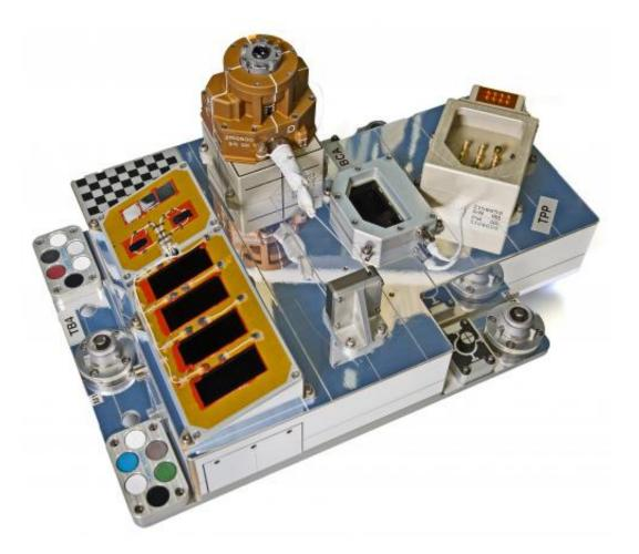
This image shows the Robotic Refueling Mission-Phase 2 task board that will be installed on the orbital outpost's Express Logistics Carrier 4. The Materials Coating Experiment can be seen on the left. Credit: NASA Goddard/Chris Gunn
