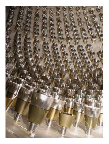
Inside the Borexino stainless steel sphere showing some of the photomultipliers used to detect the pp neutrino. Borexino Collaboration
