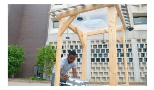
Deshawn Henry working on the water lens that can heat a liter of water to between 130 and 150 degrees Fahrenheit in a little more than an hour, destroying 99.9 percent of bacteria and pathogens.
