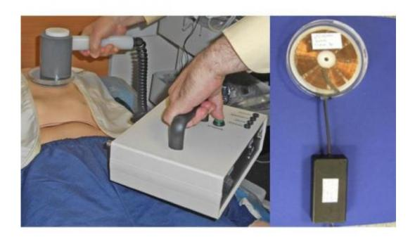
Left: The external module wirelessly receives sensor data. Right: The implantable unit, for delivering shocks
