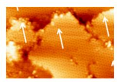
An international team of researchers has taken a significant step towards understanding the fundamental properties of the two-dimensional material silicene by showing that it can remain stable in the presence of oxygen.
