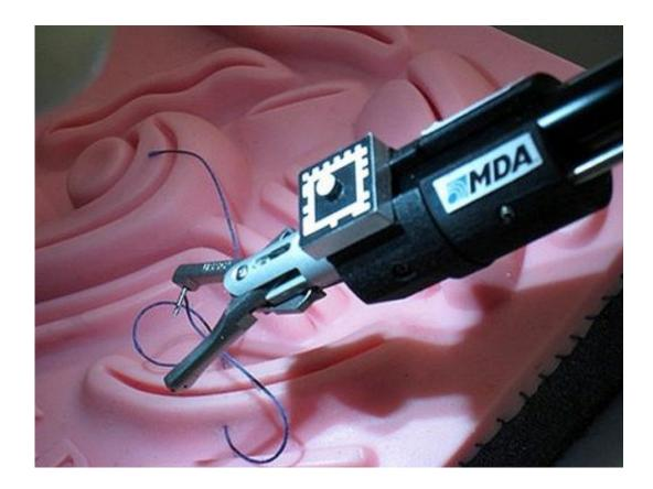
The suturing tool demonstrates image-guided anastomosis, which means the connecting of parts such as vessels. The target on the top of the tool is used to lead the tool's tip. This is the same technology used to track the robotic systems on the space shuttle and the International Space Station. Credit: MDA and CIGITI
