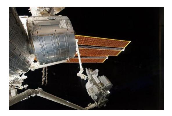
The space shuttle Endeavour's robotic Canadarm hands off the Alpha Magnetic Spectrometer-2 (AMS) to the International Space Station's Canadarm2 to complete the installation on the station's starboard truss. The Japanese Kibo complex is at left. Credit: NASA
