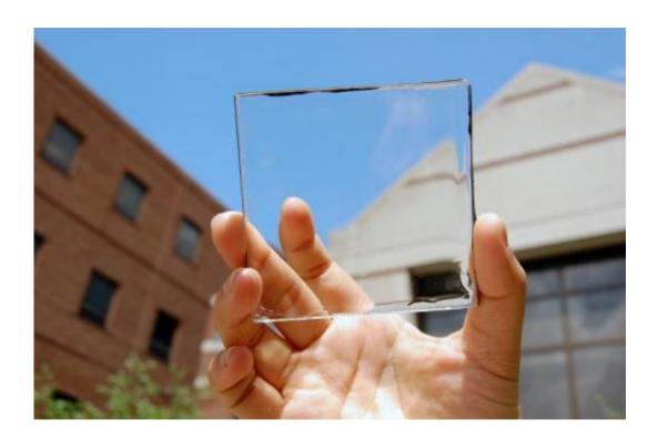
Solar power with a view: MSU doctoral student Yimu Zhao holds up a transparent luminescent solar concentrator module. Credit: Yimu Zhao.
