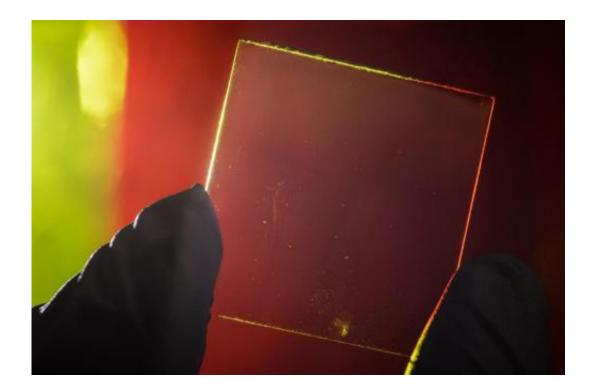
A transparent luminescent solar concentrator waveguide is shown with colorful traditional luminescent solar concentrators in the background. The new LSC can create solar energy but is not visible on windows or other clear surfaces. Photo by G.L. Kohuth.
