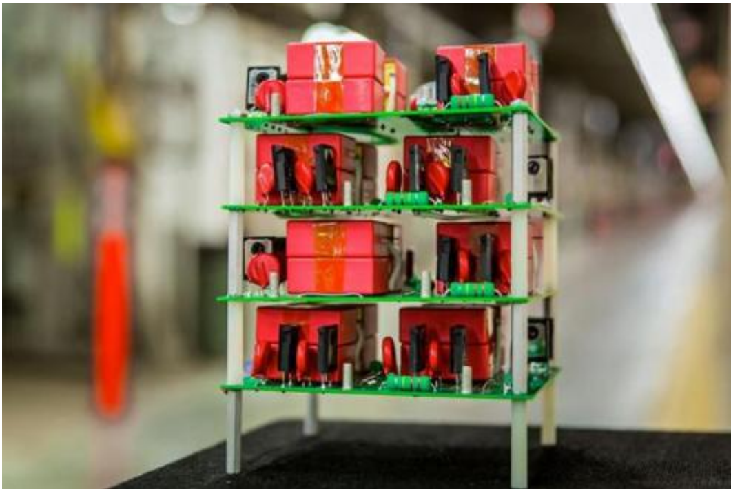
The subbooster inverse Marx modulator
