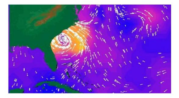
The SeaWinds scatterometer on NASA's QuikScat satellite stares into the eye of 1999's Hurricane Floyd as it hits the U.S. coast. The arrows indicate wind direction, while the colors represent wind speed, with orange and yellow being the fastest. Credit: NASA/JPL-Caltech
