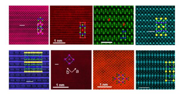
Oak Ridge National Laboratory scientists used scanning transmission electron microscopy to measure atomic-scale magnetic behavior in several families of iron-based superconductors. Credit: ORNL
