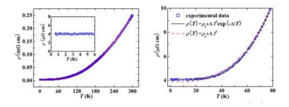
Temperature dependence of the resistivity of CrO2 film from 0.6–300 K. The solid line is the fitting result using  $\rho(T)=\rho0+AT2exp(-\triangle/T)$ . The inset is the enlarged part at low temperature; (b) A detailed comparison of fits at low temperature.
