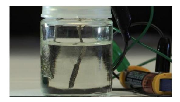
Stanford scientists have developed a low-cost device that uses an ordinary AAA battery to split water into oxygen and hydrogen gas. Gas bubbles are produced from electrodes made of inexpensive nickel and iron. Credit: Mark Shwartz/Stanford Precourt Institut for Energy
