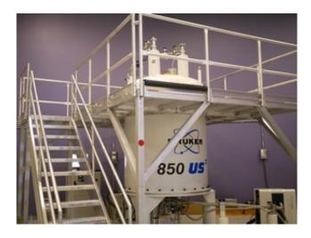
Showalter uses a nuclear magnetic resonance (NMR) spectrometer to fine-tune new methods for studying disordered proteins. Credit: Lauren Ingram
