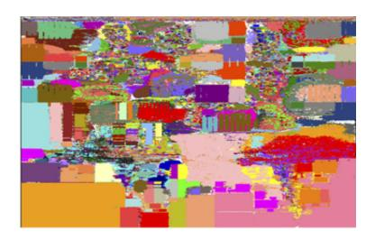
Advanced techniques such as 'structured placement,' shown here and developed by Markov's group, are currently being used to wring out optimizations in chip layout. Different circuit modules on an integrated circuit are shown in different colors. Algorithms for placement optimize both the locations and the shapes of modules; some nearby modules can be blended when this reduces the length of the connecting wires. Credit: Jin Hu, Myung-Chul Kim, Igor L. Markov, University of Michigan
