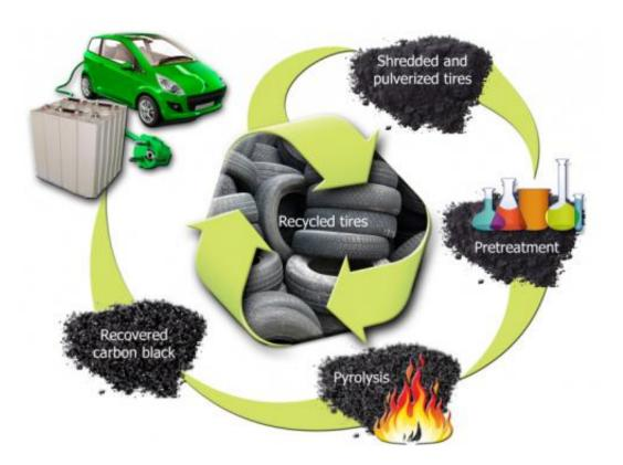
ORNL researchers' goal is to scale up the recovery process and demonstrate applications as anodes for lithium-ion batteries in large-format pouch cells. Credit: ORNL
