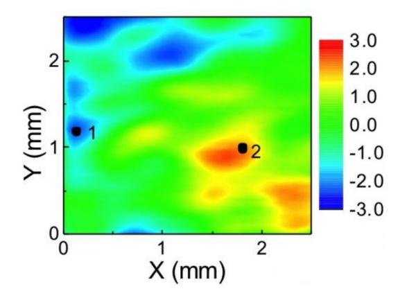
An amplitude map of terahertz radiation emitted from graphene-coated indium phosphide shows where oxygen molecules have settled on the surface after exposure to air for a few weeks. The blue at point 1 indicates high polarization due to the adsorption of oxygen molecules, while the orange at point 2 is electronically equivalent to bare indium phosphide. The research by Rice and Osaka universities makes possible a simple way to spot contaminants on graphene. Credit: Rice and Osaka universities
