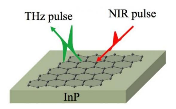
Rice and Osaka researchers have come up with a simple method to find contaminants on atom-thick graphene. By putting graphene on a layer of indium phosphide, which emits terahertz waves when excited by a laser pulse, they can measure and map changes in its electrical conductivity. Credit: Rice and Osaka universities
