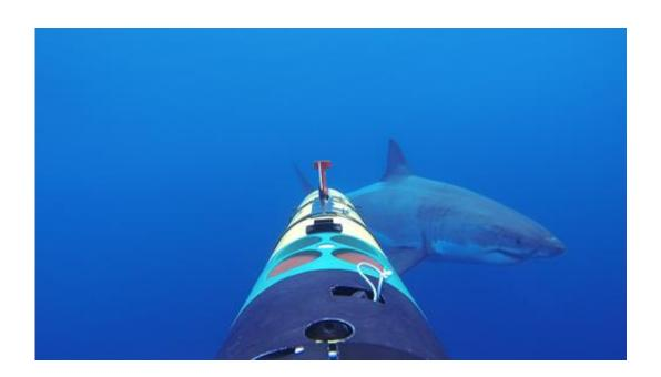
REMUS SharkCam is the first underwater robot capable of tracking and filming sharks and other marine animals up close in the wild. With six cameras total mounted on the vehicle, it recorded dramatic panoramic footage of large great white sharks attacking the underwater robot. Credit: WHOI Oceanographic Systems Laboratory
