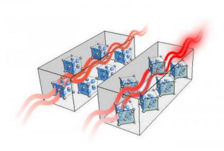
Illustration of anisotropic thermal conductivity in uranium dioxide. Scientists are studying the thermal conductivity related to the material's different crystallographic directions, hoping to improve our understanding of uranium dioxide efficiency as reactor fuel.
