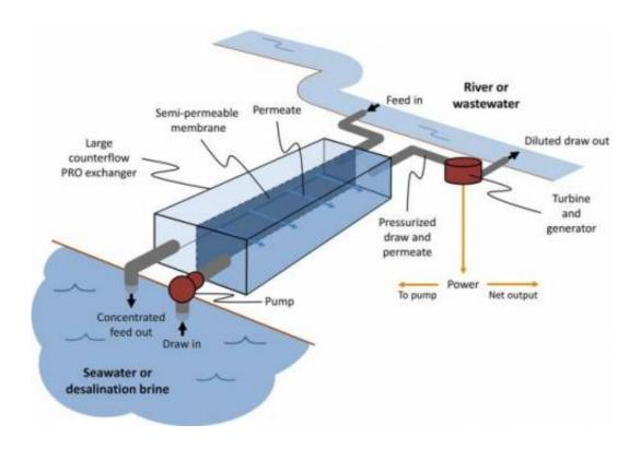
In this simplified PRO system, permeate from a dilute feed stream enters a concentrated draw stream in a pressurized state via osmosis — after which useful power can be extracted from the draw-permeate mixture. Credit: Leonardo Banchik
