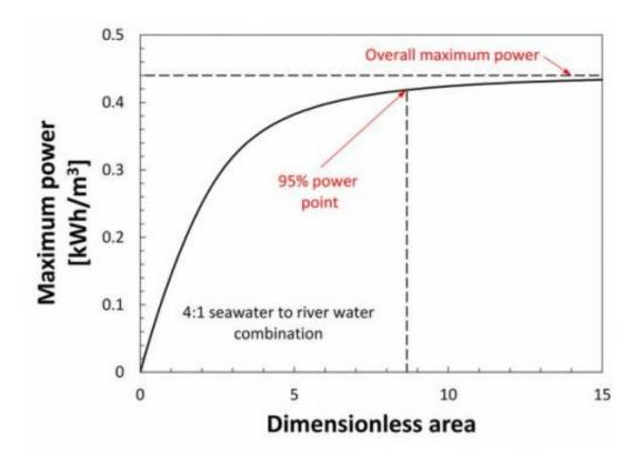
Shown here is the maximum power that can be produced for a 4:1 seawater to river water combination. As the dimensionless area gets very large, the overall maximum power can be produced. Credit: Leonardo Banchik
