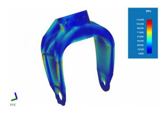
A screenshot of Akselos' software running in a Web browser for 2.01x. This app shows the stresses in the landing gear for a solar-powered airplane. Credit: Courtesy of Akselos
