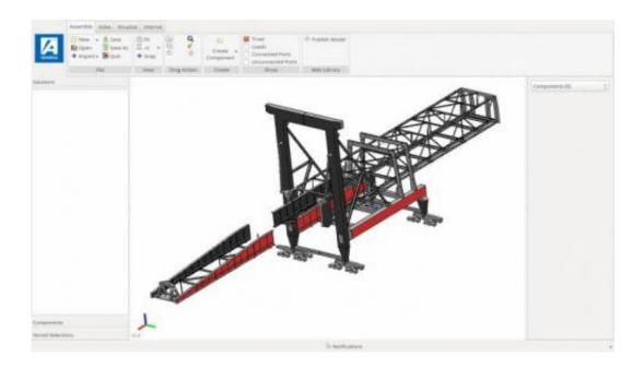
A screenshot of component-based assembly of the model of shiploading infrastructure. Credit: Courtesy of Akselos
