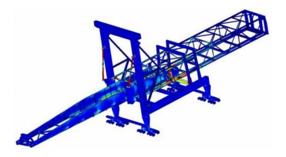
The simulation result, showing contours of the stress, for the shiploading infrastructure. Credit: Courtesy of Akselos
