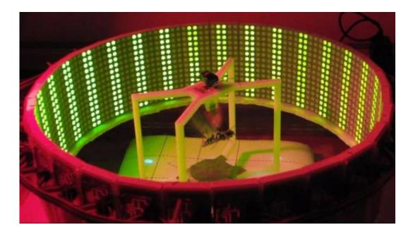
The moth is connected to a wireless platform that collects the electromyographic data as the moth moves its wings. To give the moth freedom to turn left and right, the entire platform levitates, suspended in mid-air by electromagnets. Credit: Alper Bozkurt
