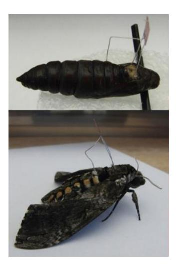
Researchers attach electrodes to a moth during its pupal stage, when the caterpillar is in a cocoon undergoing metamorphosis into its winged adult stage. By attaching electrodes to the muscle groups responsible for a moth's flight, the researchers are able to monitor electromyographic signals -- the electric signals the moth uses during flight to tell those muscles what to do. Credit: Alper Bozkurt
