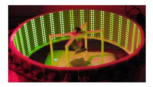
The moth is connected to a wireless platform that collects the electromyographic data as the moth moves its wings. To give the moth freedom to turn left and right, the entire platform levitates, suspended in mid-air by electromagnets. Credit: Alper Bozkurt
