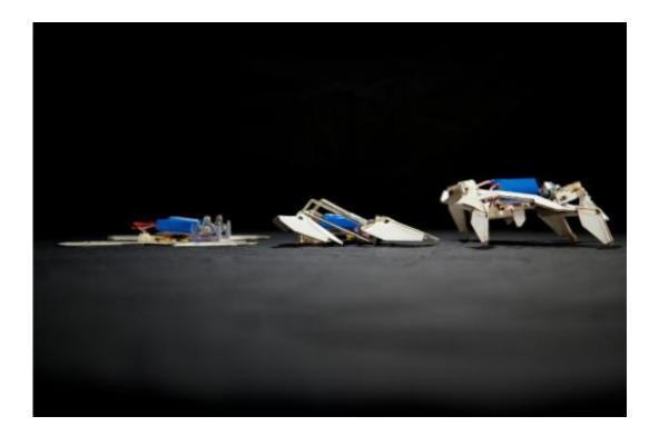
A team from Harvard's Wyss Institute, Harvard's SEAS, and MIT built an autonomous robot that starts out as a single composite sheet programmed to fold itself into a complex shape and crawl away without any human intervention. Credit: Harvard's Wyss Institute
