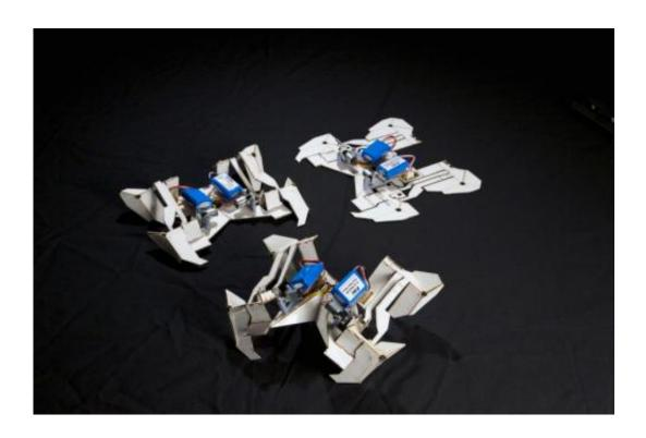
The self-folding crawling robot in three stages. Credit: Seth Kroll, Wyss Institute
