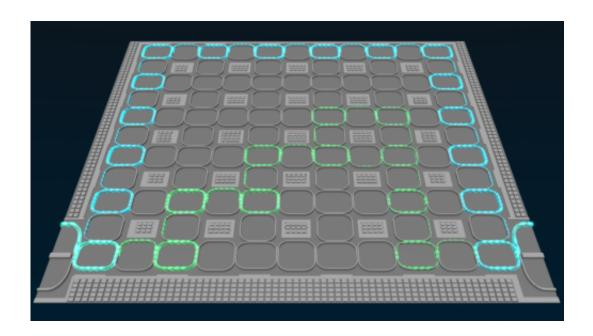
Light enters a two-dimensional ring-resonator array from the lower left and exits at the lower right. Light that follows the edge of the array (blue) does not suffer energy loss and exits after a consistent amount of delay. Light that travels into the interior of the array (green) suffers energy loss. Credit: Sean Kelley/JQI
