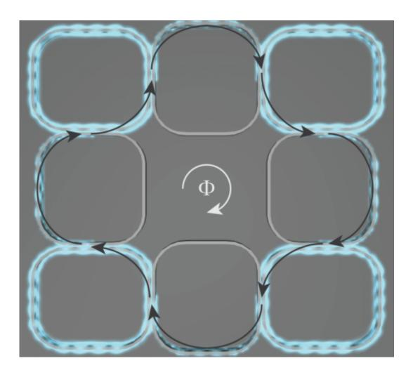
The 2D array consists of resonator rings, where light spends more time, and link rings, where light spends little time. Undergoing a circuit around a complete unit cell of rings, light will return to the starting point with a slight change in phase, phi. Credit: Sean Kelley/JQI
