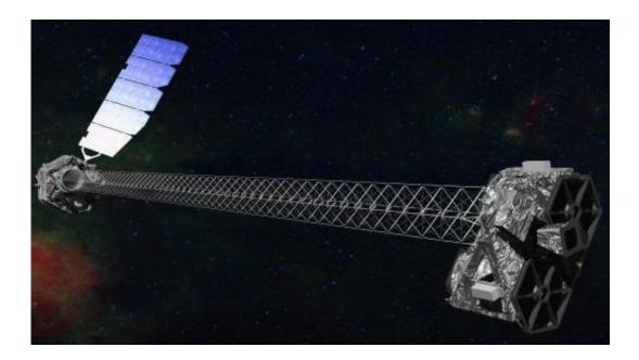
Artist's concept of NuSTAR on orbit. NuSTAR has a 10-m (30') mast that deploys after launch to separate the optics modules (right) from the detectors in the focal plane (left). The spacecraft, which controls NuSTAR's pointings, and the solar panels are with the focal plane. NuSTAR has two identical optics modules in order to increase sensitivity. The background is an image of the Galactic center obtained with the Chandra X-ray Observatory. Credit: NASA/JPL-Caltech
