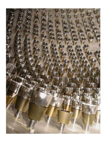
Inside view of the Borexino stainless steel sphere before nylon vessel installation and fluid filling. The sphere is 13.7 meters in diameter. The curvature and the tightly packed photomultiplier tubes (PMTs) can be seen. There are 2212 installed PMTs, most of which equipped with aluminium light concentrators to focus their view on the central volume of the detector. Optical fibres used for
