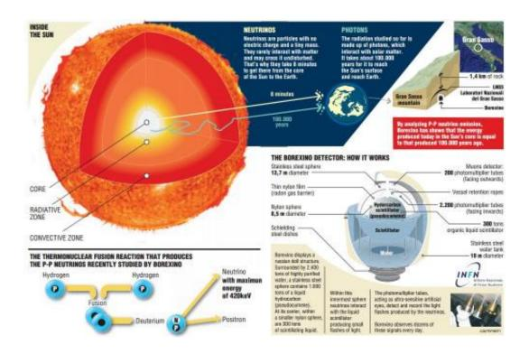
Indeed, it is the only detector on Earth capable of observing the entire spectrum of solar neutrino simultaneously. Neutrinos come in three types, or "flavors." Those from the Sun's core are of the "electron" flavor, and as they travel away from their birthplace, they oscillate or
