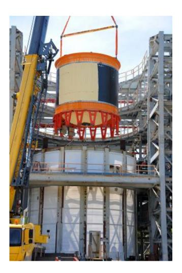
One of the largest composite cryotanks ever built recently completed a battery of tests at NASA's Marshall Space Flight Center in Huntsville, Alabama. The tank was lowered into a structural test stand where it was tested with cryogenic hydrogen and structural loads were applied to simulate stresses the tank would experience during launch. Credit: NASA/David Olive
