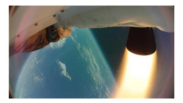
In this June 28, 2014 video frame provided by NASA, rockets fire on NASA's Low-Density Supersonic Decelerator (LDSD) as the saucer-shaped test vehicle flies into near-space. NASA engineers insist that a test of technology they hope to one day use above Mars achieved most of its objectives and taught them essential lessons for their next try despite a parachute that virtually disintegrated the moment it deployed. (AP Photo/NASA)
