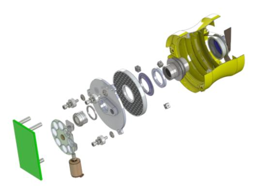
This is an exploded view of the CubeSat-class 50-millimeter (2-inch) imaging instrument that technologist Jason Budinoff is manufacturing with 3-D-printed parts. It shows the mirrors and integrated optical-mechanical structures. Credit: NASA Goddard/Jason Budinoff
