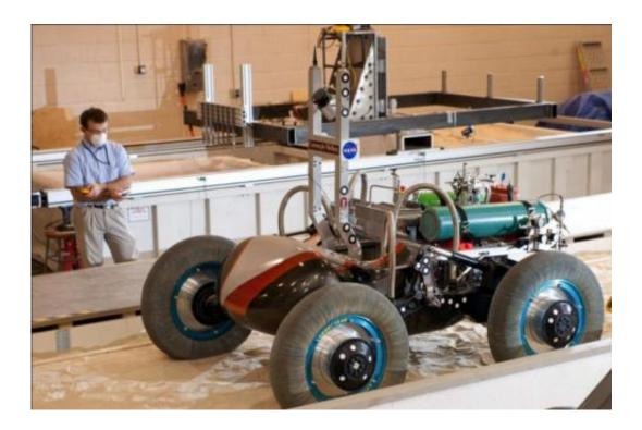
The Scarab lunar rover is one of the next generation of autonomous robotic rovers that will be used to explore dark polar craters at the lunar south pole. The rover is powered by a 100-watt fuel cell developed under the Space Power Systems Project under Game Changing Development program. Supported by NASA, the rover is being developed by the Robotics Institute of Carnegie Mellon University. Image Credit: Carnegie Mellon University
