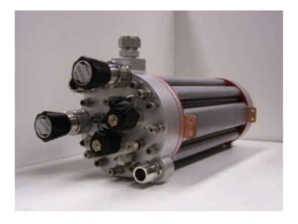
A model of a 3-kilowatt fuel cell that could be used for deep space power applications. Credit: NASA
