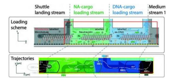
The assembly carrier moves through several reaction chambres where different molecules bind to its surface. The graph below shows the trajectory of a single shuttle. Credit: from Steuerwald et al. 2014
