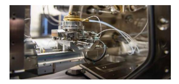
What makes the Scios tool a game changer? It allows biologists to nanomachine cells to reduce them to the thickness required for electron microscopy without creating any sample distortions and while maintaining cryogenic temperatures.
