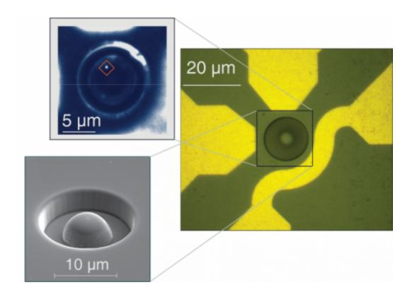
These images show a diamond sample with a hemispherical lens (right and lower left), and the location of a single electron spin/quantum state visible through its light emission (upper left). The scale bar on the image at upper left measures five microns, the approximate diameter of a red blood cell. Credit: Courtesy of Awschalom Lab/University of Chicago
