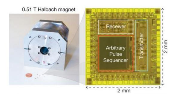
The small chips could be used in a portable spectrometer for on-demand applications in the field. Alternatively, they could be assembled in parallel to perform high-throughput NMR spectroscopy, dramatically accelerating molecular analysis in the laboratory. Credit: Dongwan Ha, Harvard SEAS
