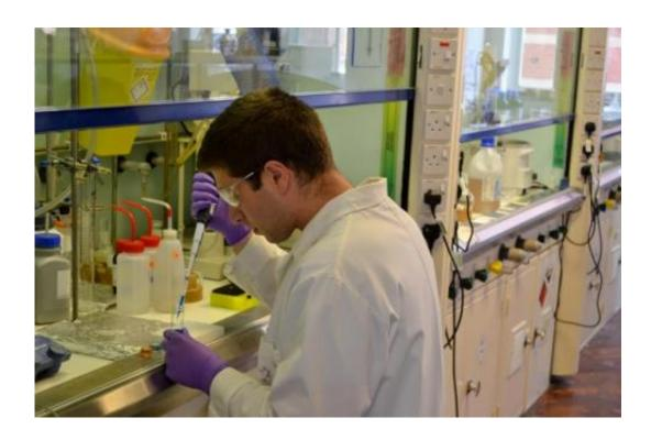
George Karageorgis prepares reaction arrays: 96 different reactions can be quickly tested in a plate the size of a DVD. Credit: Steven Kane / University of Leeds
