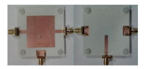
The prototype device operates as a filter and an antenna simultaneously.
