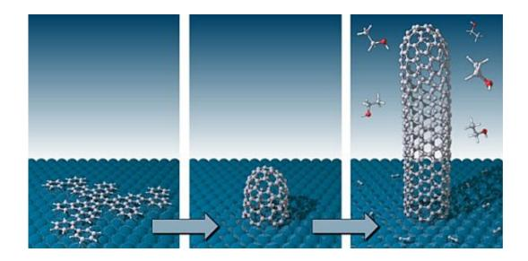
On a Platinum surface, the planar hydrocarbon precursor folds into an end cap, that in turn acts as seed for the growth of a well-defined carbon nanotube. Credit: Empa / Juan Ramon Sanchez Valencia
