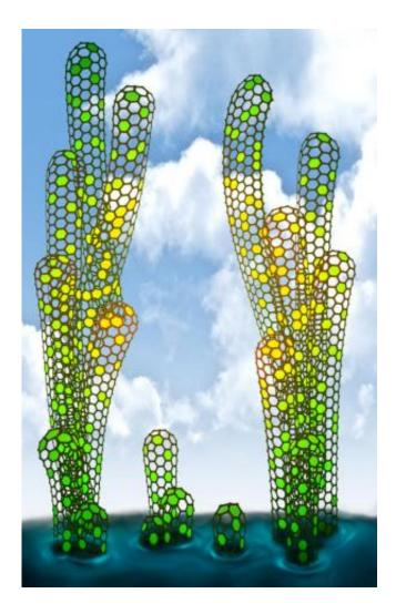
Selective growth of (6,6) single-walled carbon nanotubes on a Platinum surface. Tiny caps folded from a planar molecular precursor act as seeds for the growth of well-defined nanotubes by the incorporation of carbon from a gas such as ethanol or ethylene. Credit: Empa / Universität Erlangen / Konstantin Amsharov
