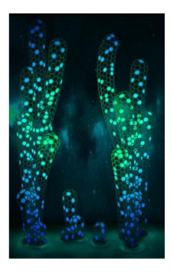
Selective growth of (6,6) single-walled carbon nanotubes on a Platinum surface. Tiny caps folded from a planar molecular precursor act as seeds for the growth
