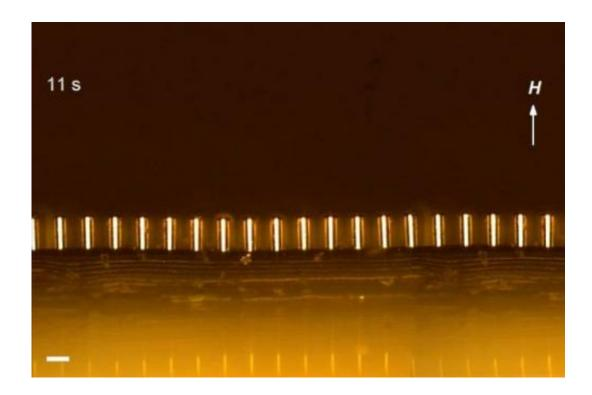
The new material designed by MIT researchers is a flexible polymer "skin" coated with microhairs (white lines) that tilt in response to a magnetic field.
