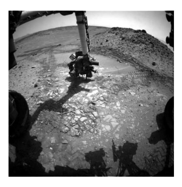
This image from the front Hazcam on NASA's Curiosity Mars rover shows the rover's drill in place during a test of whether the rock beneath it, "Bonanza King," would be an acceptable target for drilling to collect a sample. Subsequent analysis showed the rock budged during the Aug. 19, 2014, test. Credit:
