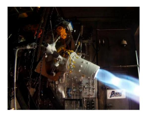
Purdue students have conducted the first "hot-fire" test of the rocket, which uses liquid oxygen and liquid methane propellants. The students have designed, built and tested a central part of the new engine - called the thrust chamber or combustor - as part of NASA's Project Morpheus. Credit: Purdue University
