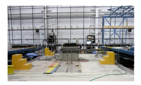
Pipeline specimens were anchored to shake tables to simulate the passage of a seismic wave through two adjacent push-on joints. Experiments took place at a University at Buffalo laboratory. Credit: NEES
