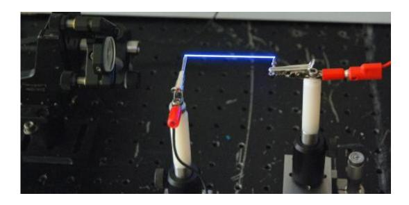
Miniature lightning: The team used a femtosecond laser to create a thin column of plasma – a special charged state of matter – in the air between two electrodes. Credit: Pavel Polynkin
