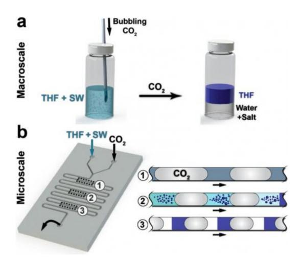
Phase separation of a switchable water solution occurring (a) at the macroscale and (b) in a microfluidics reactor. Credit: Lestari, et al. ©2014 American Chemical Society
