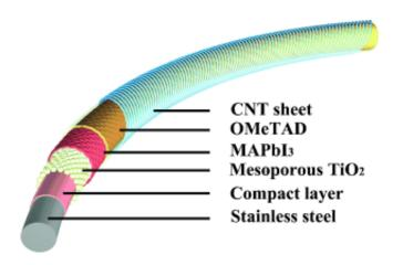
(Phys.org) —Textile solar cells are an ideal power source for small electronic devices incorporated into clothing. In the journal *Angewandte Chemie*, Chinese scientists have now introduced novel solar cells in the form of fibers that can be woven into a textile. The flexible, coaxial cells are based on a perovskite material and carbon nanotubes; they stand out due to their excellent energy conversion efficiency of 3.3 % and their low production cost.
