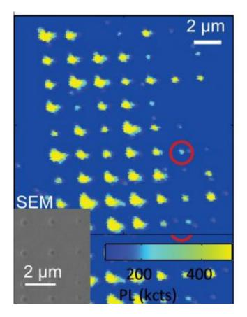
A surface confocal scan of a diamond sample shows the NV centers in yellow. A single NV center is circled in red. The inset scanning electron microscope image shows holes in a separate sample as tiny dimples. Credit: F.J. Heremans and D. Awschalom/U. Chicago and K. Ohno/UCSB
