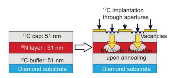
This is a schematic of the process to localize NV centers in 3-D. The researchers blasted carbon ions through holes to create vacancies and heated the diamond to make the vacancies mobile within the crystal. NV centers could form in the nitrogen-doped layer below where the holes were placed. Credit: F.J. Heremans and D. Awschalom/U. Chicago and K. Ohno/UCSB
